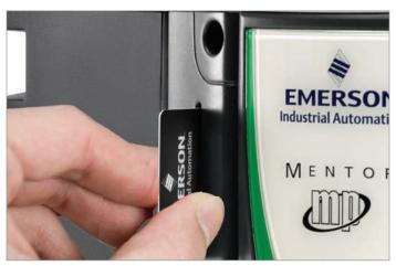
The SmartCard memory device supplied with every MP drive can be used to back up parameter sets and PLC programs and copy them from one drive to another.
