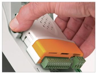
Commander SK drive models size B and up can be ordered with a snap-in SM-I/O-LITE Option Module. This module provides control over additional pump application parameters. Additional features include:
